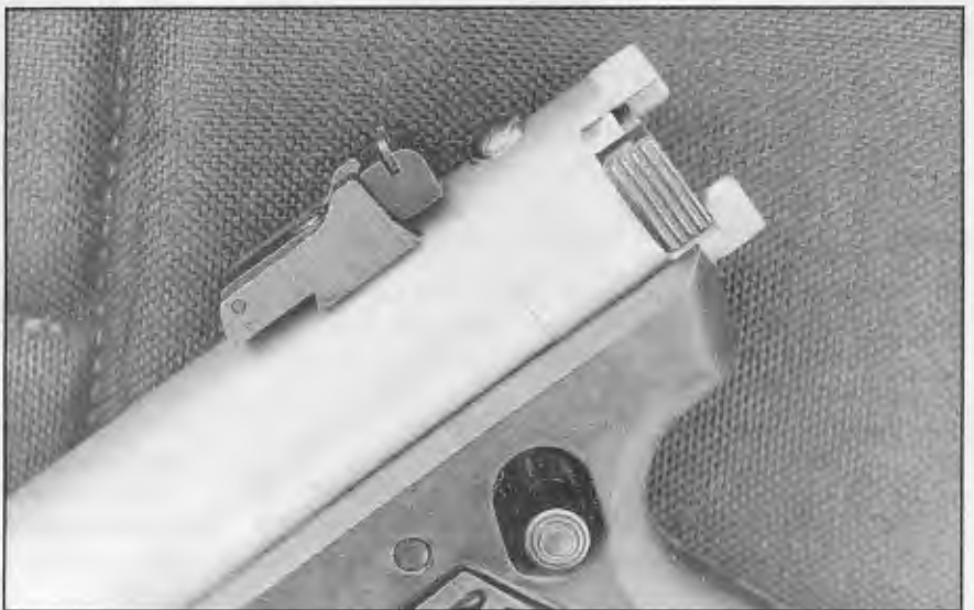
Government-issue Arms Tech sound-suppressed Ruger 22/45 pistols are equipped with a bolt lock in the form of a sleeve at the end of the receiver tube. When rotated 10 degrees clockwise it will block the bolt to further reduce the sound pressure level and will also prevent the ejection of empty cases.
